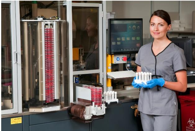
distribution agreement for COPAN WASP®: Walk-Away Specimen Processor with Thermo Fisher Scientific Inc. in the United States. The COPAN WASP® provides a total solution for pre-analytical microbiology specimen processing with a robust modular system able to automatically plant and streak plates, prepare gram slides, apply susceptibility disks, and inoculate broths.
